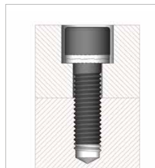
Countersunk socket head bolt secured in position
